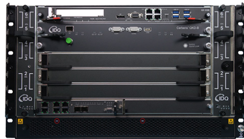
The Cerberis 3 QKD System, in ATCA chassis
