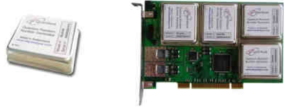
Figure 3: The Quantis random number generator, available for example as an OEM component (left) and as a PCI-card (right), offers high-quality random numbers at a speed of up to 16 Mbits/sec.
