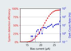
SDE and dark count rate measurement of an IDQ SNSPD, as a function of the applied bias current, tested at 1550 nm.
