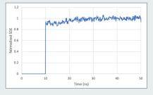
Recovery time measurement of an 8-pixel Parallel SNSPD, tested at 1550 nm.
