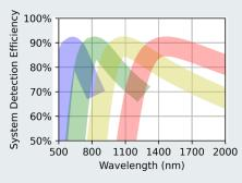
Approximate expected spectral response for four cavity designs. Max efficiency depends on detector grade
