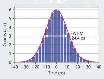
Timing jitter measurement of a standard IDQ SNSPD at 1550 nm, recorded with an ID1000 Time Controller. The plot shown is the raw data, including all instrument jitter contributions. The contribution of the SNSPD is less than 22.3 ps FWHM.
