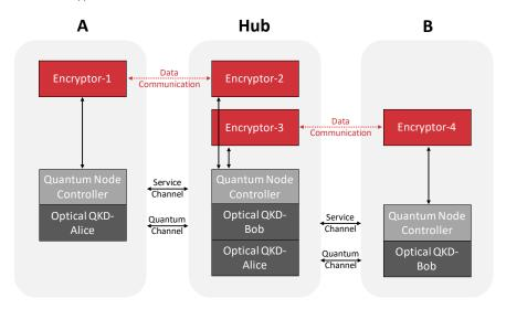
The two 5G nodes are connected through a network Point of Presence defined as a Hub (H) for the encryption and QKD design as shown on the diagram explaining the components of this use case.
