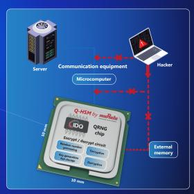
\*Q-HSM = Quantum Hardware Security Module
