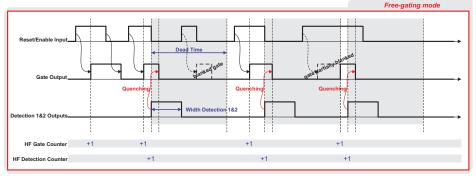
A two-channel event counter and a coincidence counter as an auxiliary independent block.
