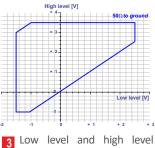
voltage ranges when the output is loaded at  $50 \Omega$  to ground.
