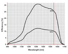
1 Efficiency versus wavelength at 10% and 25% levels ( $\lambda$ =1550 nm)
