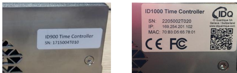
Figure 4: Sticker on the rear panel of the Time Controller device, printed with the serial number only (ID900, left image) or with both the serial number and IP address (ID1000, right image)
